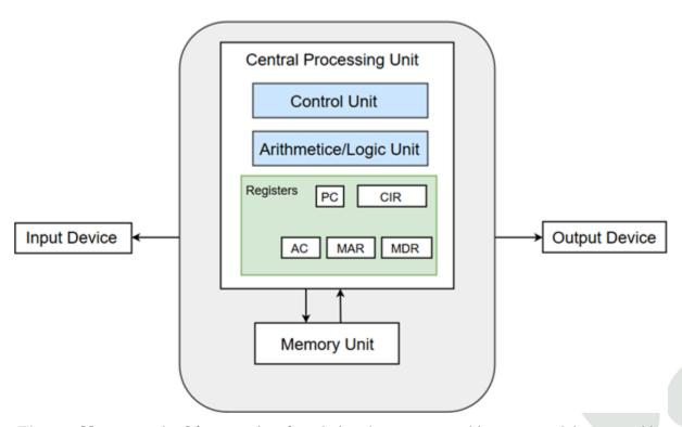
The **von Neumann Architecture** is a foundational computer architecture model proposed by **John von Neumann** in 1945. It serves as the basis for most modern computers, where a single memory system is used to store both **instructions (programs)** and **data**.
